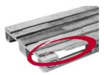
• One board is diagonally or transversely broken off.
